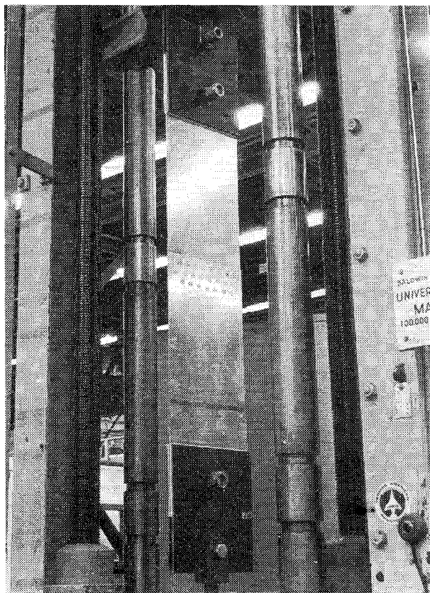
Fig. 7 An ultrasonically spot welded single overlap joint between 12 x 30 x 0.063-in.-thick panels of 7075-T6.
